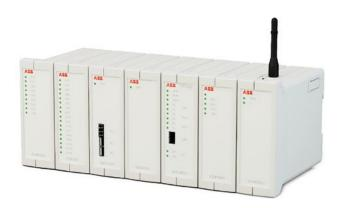
Distribution automation product for power grids. Interface with your SCADA to obtain a complete understanding of the status of your grid on a distribution level with RTU520.
