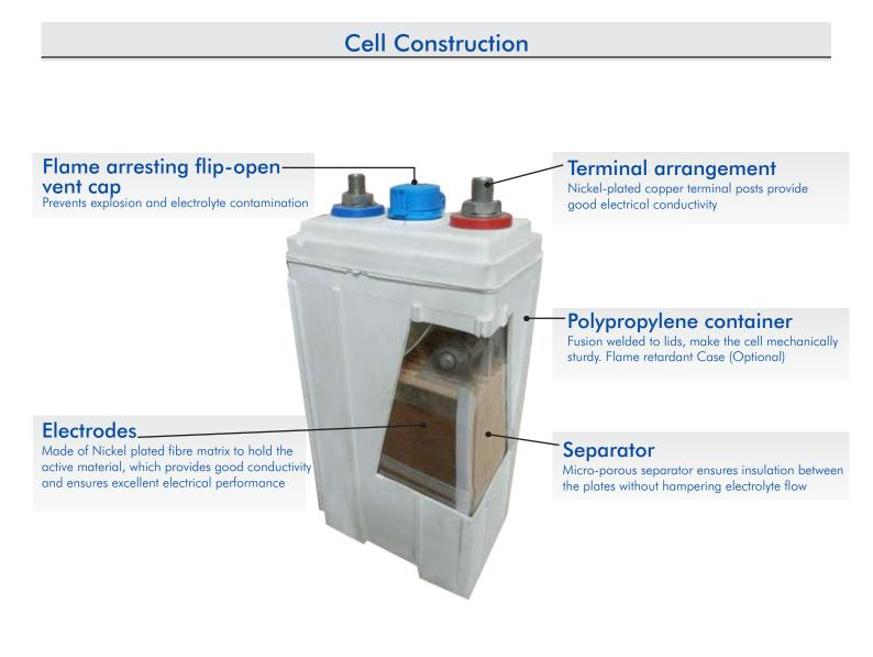
These batteries are built in polypropylene containers to which lids are thermally welded to withstand impact resistance. This type of cells are translucent in nature, so electrolyte levels can be visualized. Flame retardant containers in the other hand are Opaque in nature, so the levels of electrolyte is not visible. If requested by the customer, flame retardant cells can be offered.
