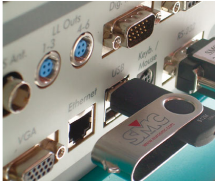
Low Level Outputs, USB and Ethernet connections
